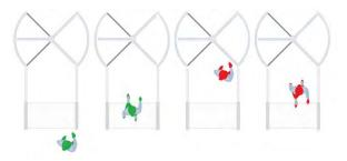
Present authorized credentials, pass through metal detector with metal, turnstile remains locked and alarm sounds.
